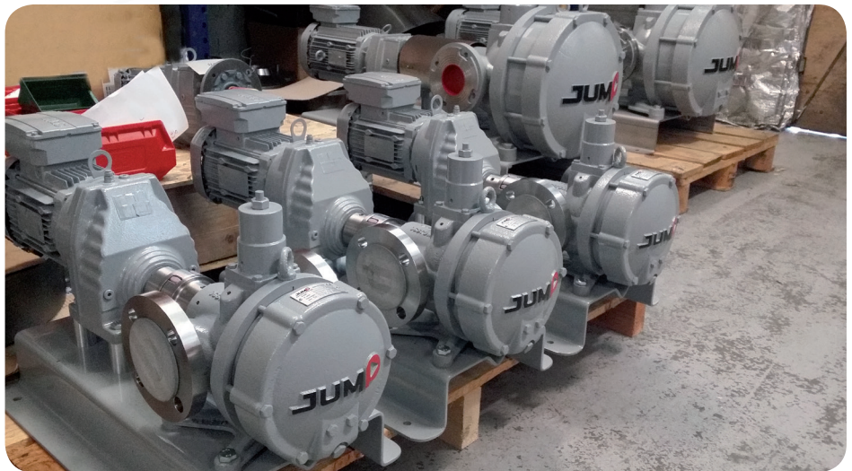
JE5c and JE36c pumping units on stationnary chassis
