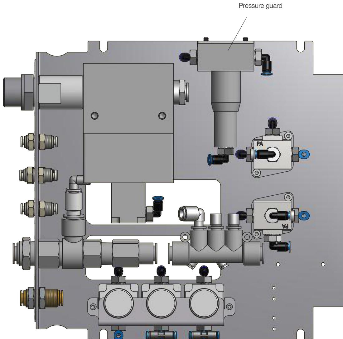
If the incoming air pressure changes, or if the load falls when the air pressure is lost, it may be necessary to adjust the pressure switch.
